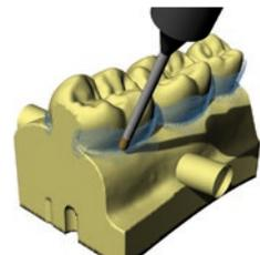
Automatic 5-Axis Undercuts Machining
