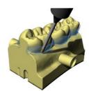
Automatic 5-Axis Undercuts Machining
