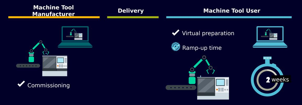
Essentially shorten the commissioning time at the final destination based on preparation on a virtual model
