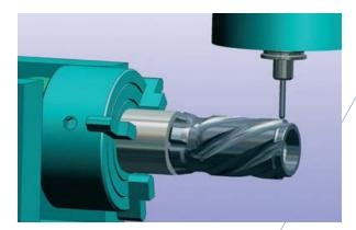
So, as part of the 5-axis project, dedicated functionality was developed to find 5-axis features on a solid model. Easy to use dialogs were created to allow complex 5-axis techniques to be used without becoming a 5-axis machining expert. High quality, full machine simulation was included to allow clear visualization of the machine movement. And finally, extra effort was put in to provide a strong solution for 5-axis on turning centres.
